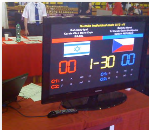
Picture 8: Example of LCD monitor showing software scoreboard
